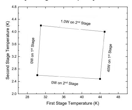
Typical\* Cooling Capacity at 4.2K and 45K vs. Input Power Frequency and Input Power
